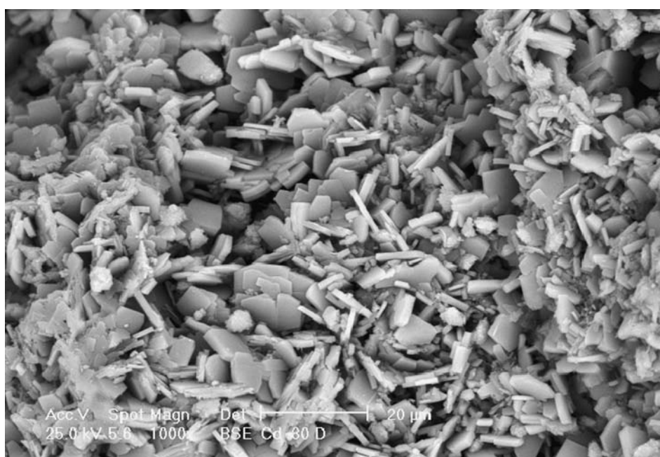
Figure 1. SEM image of zeolitic rock treated with 0.002 M \text{Cd}(\text{NO}_3)_2 solution for 48 h at 303 K.
